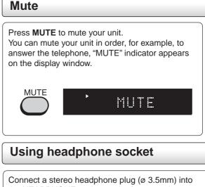
Connect a stereo headphone plug (ø 3.5mm) into the HEADPHONE socket on the front panel. The speakers are automatically disconnected when you plug in the headphones (not supplied).
